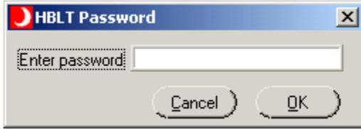
This panel allows the operator to enter the HBLT password for the delete test, new test and update test functions on the HBLT Test Parameters panel. Each time the HBLT Test Parameters panel opens, Pressure Manager resets the password to no characters.
