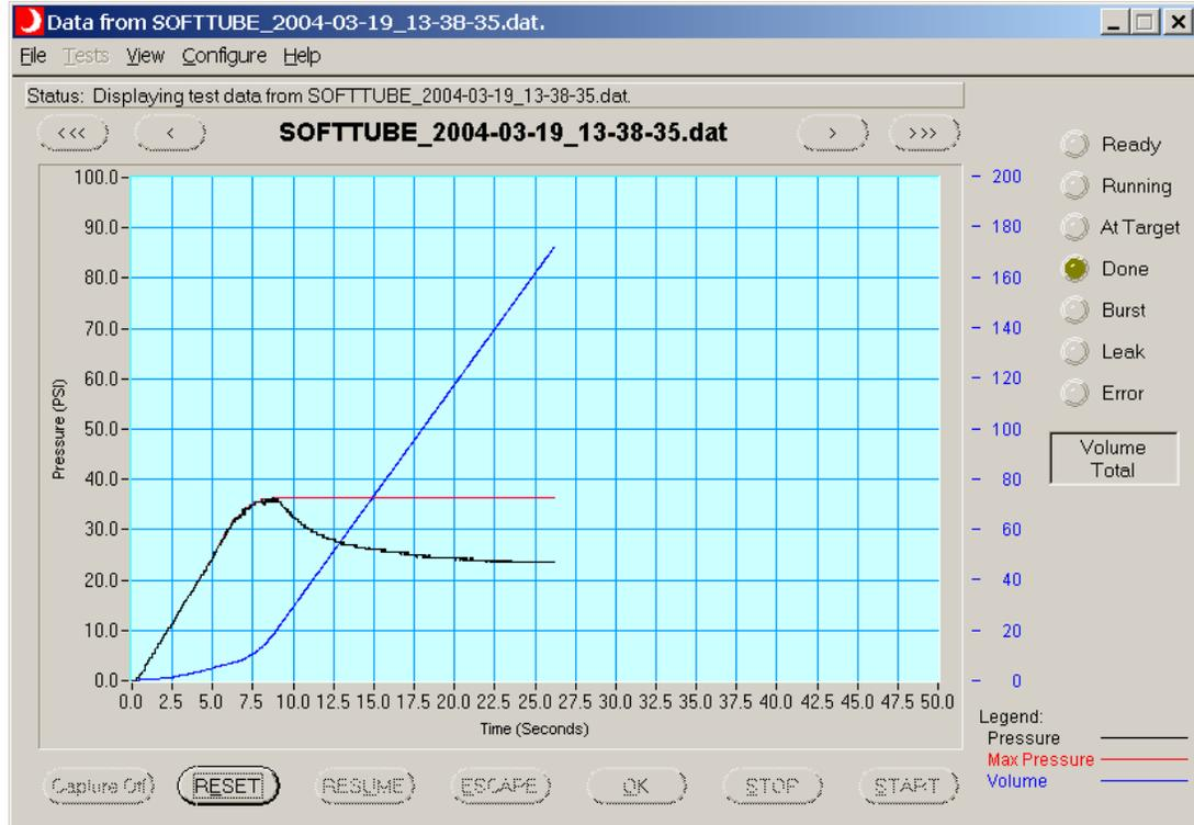
This is the main Pressure Manager panel. Use the main menu to select special functions and to open the other panels. Use the buttons located at the bottom of the panel to control a test's execution. Use the top buttons to scroll the strip chart data after a test completes.
