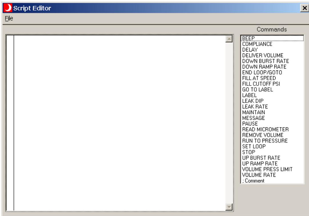
Use this panel to enter a new script or edit an existing script. The editor is content directed. That is the editor knows the syntax of the available script commands. The editor validates and completes the command syntax while the operator keys in new lines. The editor also checks parameter values based on HBLT pressure type and model type. In short, the editor insures that the operator enters only correctly formatted scripts.
