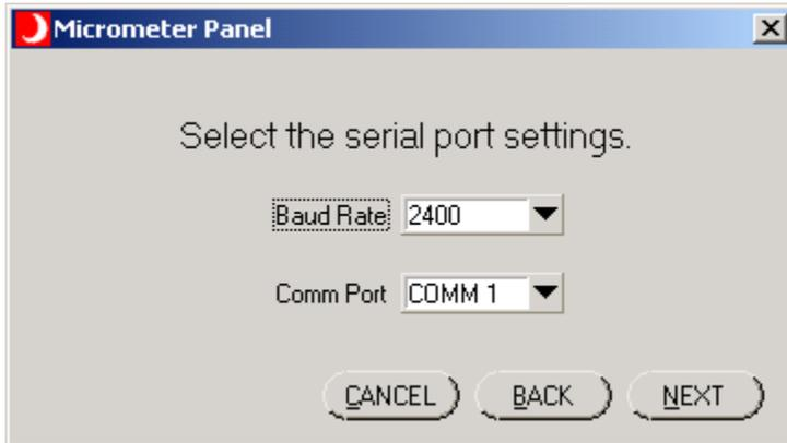
Use this panel to select baud rate and comm port for the Mitutoyo and Keyence serial interfaces.
