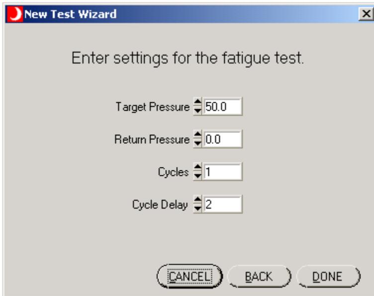
Use this panel to enter the parameters specific to the fatigue test.
