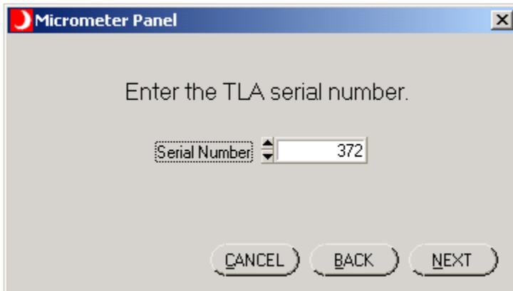
Use this panel to enter the TLA serial number located on the side of the laser head.
